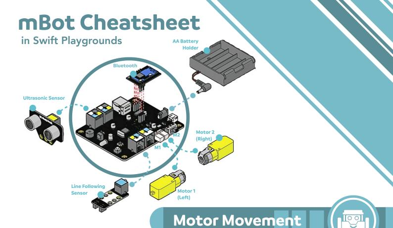
Motors can go forward or backward using positive or negative numbers.
